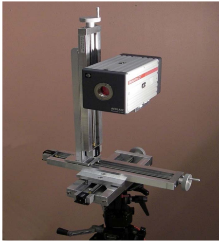
Fig. 3 The high speed video camera mounted on a x, y, z positioning stage that is equipped with micrometers
